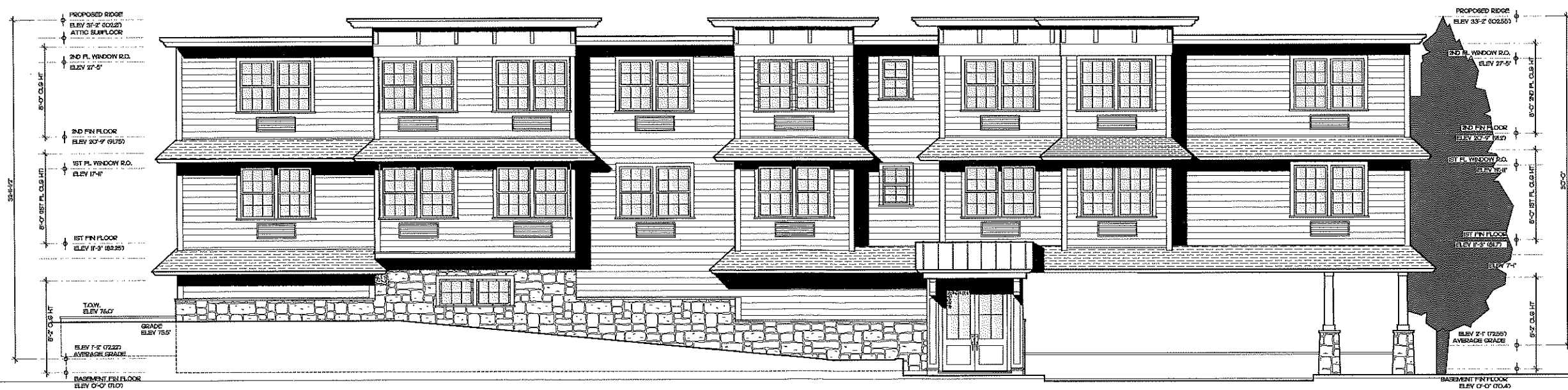
3 ALTERNATE FRONT MAIN STREET ELEVATION - FLAT ROOF 3/16" = 1'-0"
